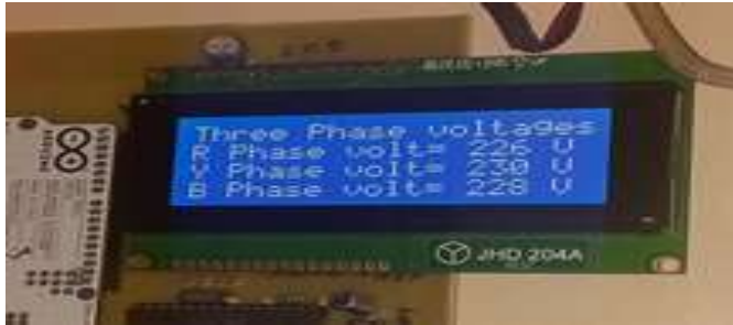
Figure 10. LCD Phase voltage value display
