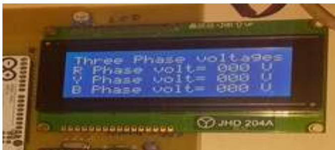
Figure 12. LCD showing loss of supply from all three phases
