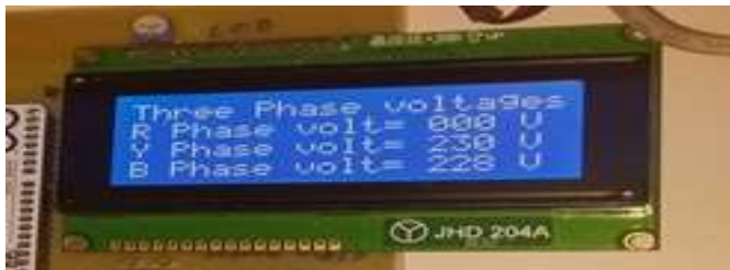
Figure 11. LCD showing loss of supply in red phase
